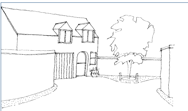
Fig 6.4: Including a flat over the garage (FOG) provides a small dwelling that helps meet Neighbourhood Plan policy, and also increases security by providing overlooking of the courtyard. Including trees and good quality paving creates a good quality setting for the flat.
