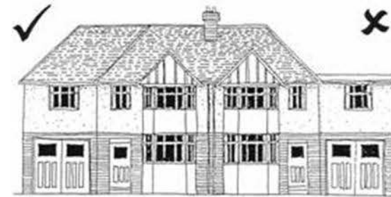
Figure 2 Pitched roof extensions will be encouraged
