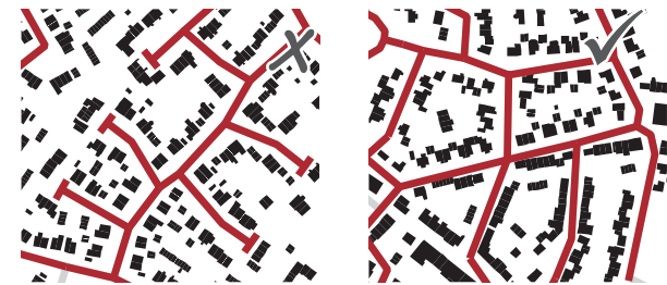
Fig 8.4: Left - avoid a layout based on dead-ends Right - a connected layout of streets is much easier to access on foot or by bike
