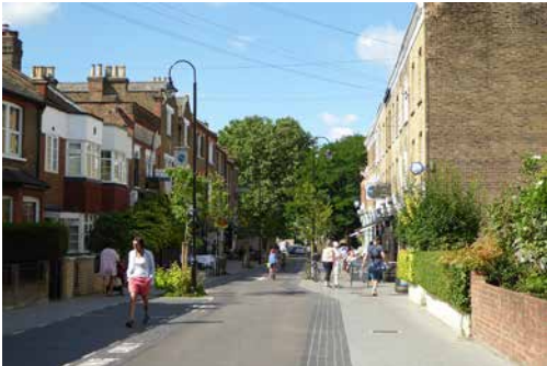
Orford Road, Waltham Forest, London closes a local centre street to cars. The street surface is kept at grade but segmented by texture changes to increase ease of movement and legibility.
