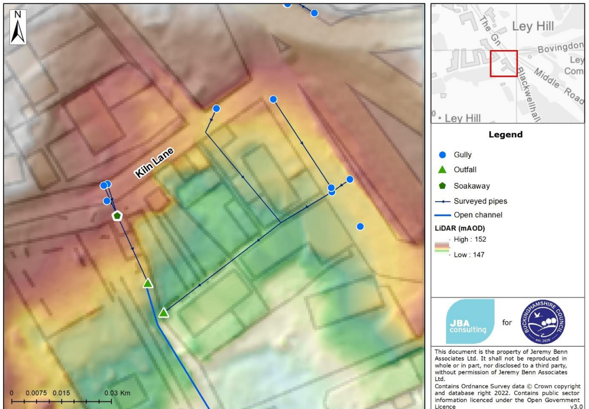
Figure 3-2: Surveyed highway drainage near Crown Cottages
