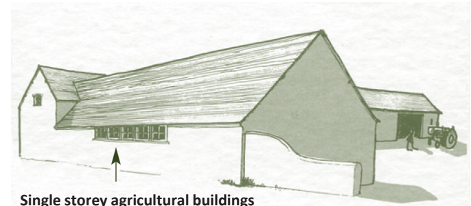
Single storey agricultural buildings are often of a linear shape - a ribbon window of traditional pattern can be appropriate
