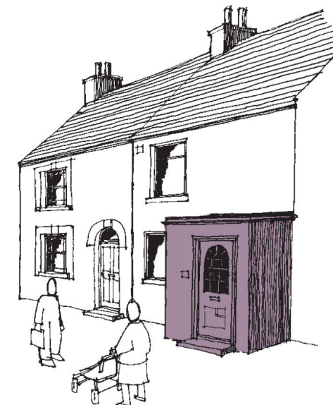
Figure 8.24: Porch design does not relate well to the shape or design of the building
