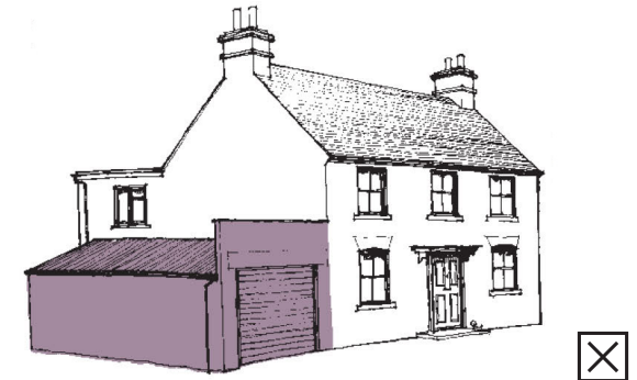
Figure 8.37: The use of parapets on garages is not encouraged. A preferred arrangement is for pitched roofs of similar form to the main roof
