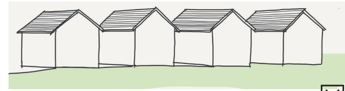
Figure 7.10: Space between buildings is inadequate
