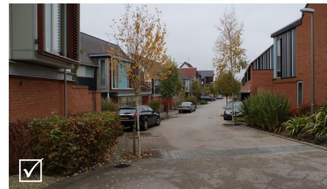
Successful shared surface street (serving local properties only) incorporating tree planting, soft landscaping and parking
