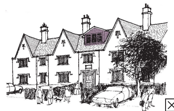
Figure 8.31: Bulky dormers of unsympathetic appearance detract from the building elevation
