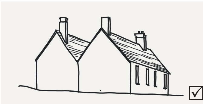
Figure 7.18: Building with twin roofs helps to reduce the impression of the overall bulk. However a central valley gutter is created which needs careful detailing.
