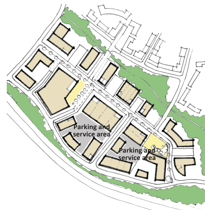
Figure 5.30: Service yards and parking should be internalised within the perimeter block to reduce impact on the street environment
