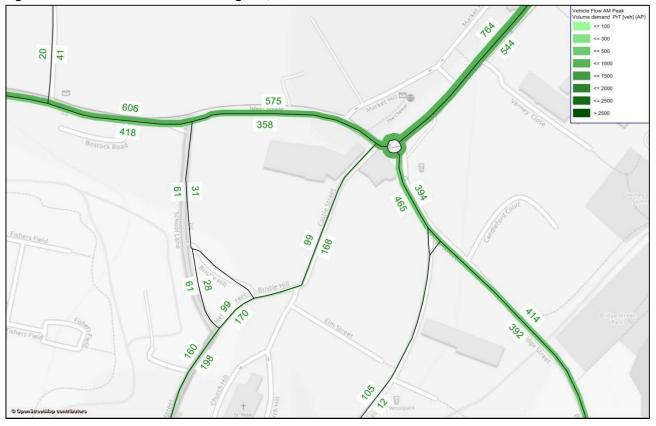
Figure 7.6: PM Peak Link Flow in Buckingham, 2013<sup>81</sup>
