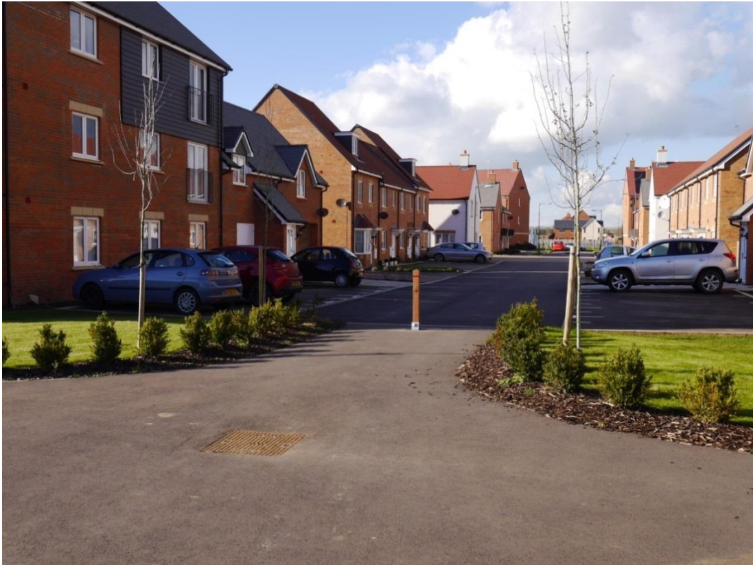
Use of filtered permeability through the site to make walking and cycling more attractive
