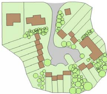
Fig 5.5d Lack of boundary definition and dominant access road within cul-de-sac development
