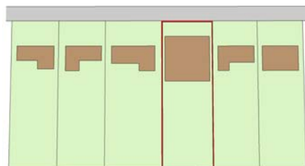
Fig. 6.2b Proposed new dwelling which adheres to technical guidelines but may appear over-dominant due to overall mass
