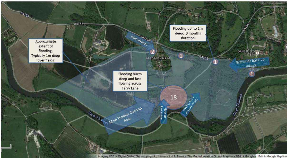
Figure 6 Location of flooding in February 2014 in Medmenham area (Millard K. and McLeish P., 2014)
