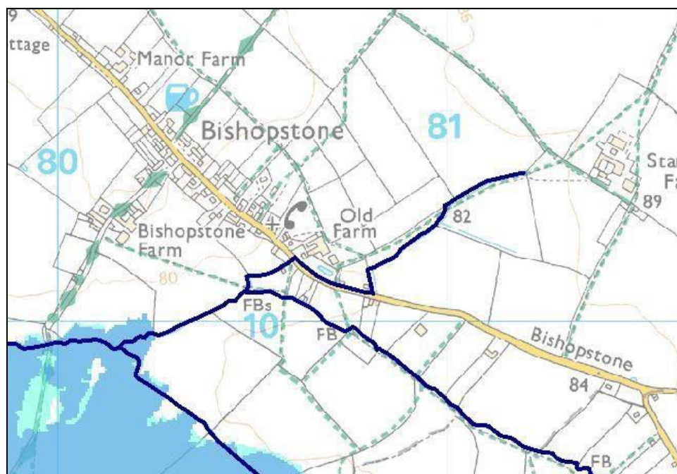
Figure 4 EA flood map showing Standall's Ditch and Scotsgrove Brook 1:100 year event (flood zone 3) in dark blue and 1:1000 year (flood zone 2) in light blue (EA, 2014)
