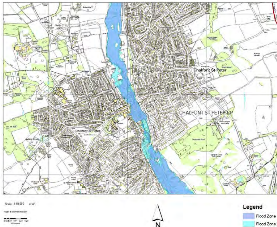
Figure 9: EA flood map showing the River Misbourne 1:100 year event (flood zone 3) in dark blue and 1:1000 year (flood zone 2) in light blue (EA, 2014) (Ordnance Survey License 100021529 2014)
